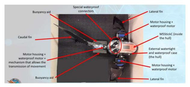
The hull, the caudal fin and the lateral fins were 3D printed as well as some minor parts of the robot. The hull is watertight thanks to its special connectors, internal O rings and special design.
