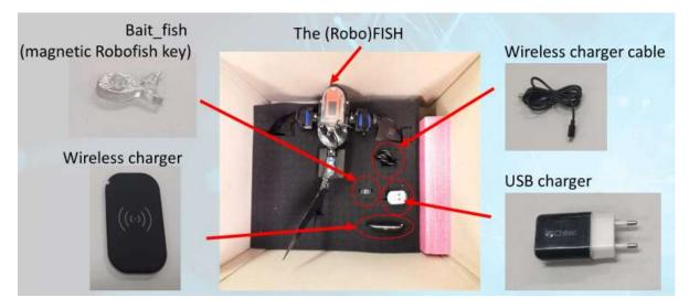
The specific parts of the main robot are the ones highlighted in the picture below:
